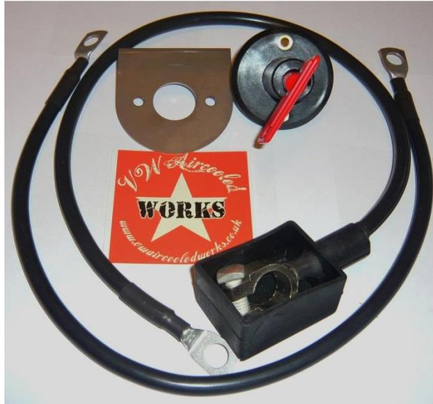
The battery isolator switch comes with the battery isolator, stainless steel mounting plate, 2 x 0.5 metres battery cable and fastenings. One cable has 10mm rings on both ends and is for connecting to the vehicle body, the other cable has a 10mm ring for connecting to the isolator and the other end connects onto the negative terminal of the battery.
