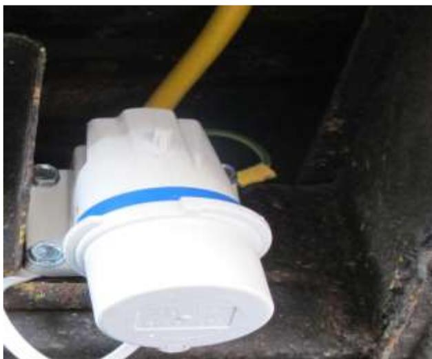
7. This completes the mains 'line in' part of the installation. The supply of power to the sockets will vary in terms of camper layout and personal preference so the following are basic outlines.
